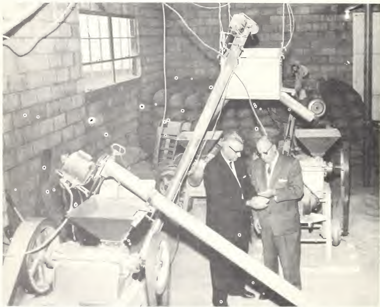
Figure 8.--Debranning wheat for the market test product by using debranning machines connected in series.
